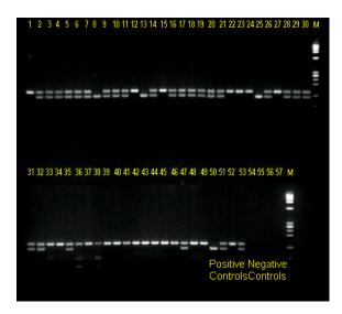
Lane 8 - FecB carrier Homozygous  $(FecB^B / FecB^B)$  at 110 bp Lane 2- FecB Heterozygous  $(FecB^B / FecB^+)$  at 140 bp and 110 bp Lane 1 - FecB non-carrier Homozygous  $(FecB^+ / FecB^+)$  at 140 bp
