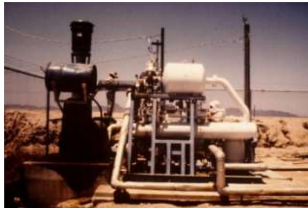
10 kW organic Rankine cycle solar thermal power plant
