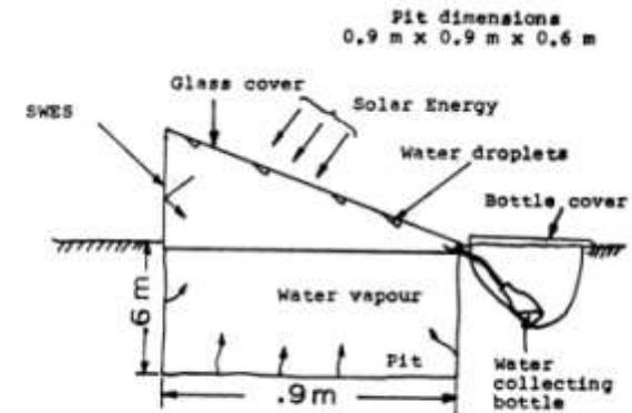
Fig. 1 Schematic of Soil Water Evaporation Still (SWES)
