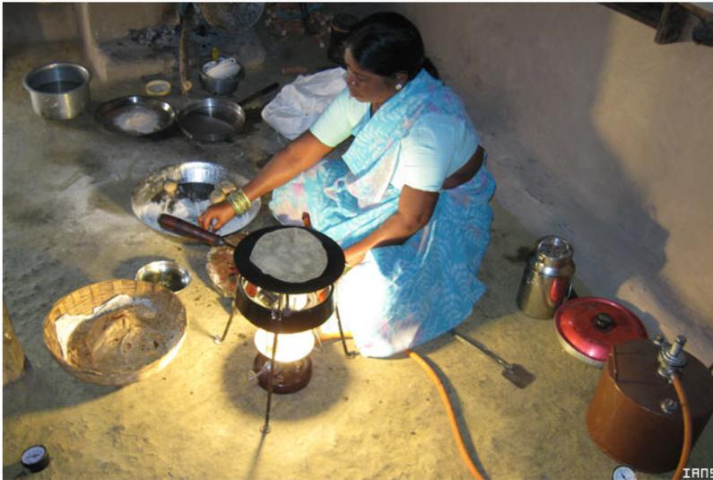
"To our knowledge, it is the first such device where both lighting and cooking are combined together resulting in tremendous energy efficiency and saving of fuel," Rajvanshi, a graduate of Indian Institute of Technology in Kanpur, said.
